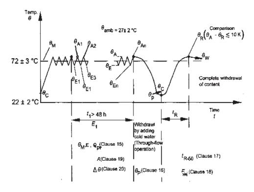
Fig. 2 Measurement of Thermal Storage Water Heaters
